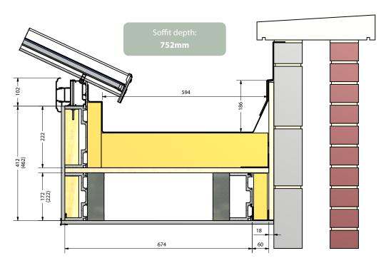
The glazed lantern is constructed using either Synseal's tried and tested K2 roof system, or the market-leading Global roof.
