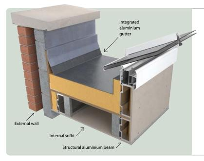
Internally a substantial plasterboard soffit 752mm in depth conceals the aluminium perimeter, primary and lantern beams and provides the classical orangery look, allowing downlighters or speakers to be integrated. The vertical face of the soffit extends right up to the underside of the glazing rafters and is 514mm in overall height, or 564mm if the deeper perimeter/primary beam is specified. A choice of internal trims can also be incorporated for a neat finish.
