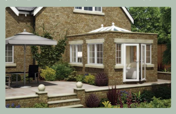
The Integra system features an insulated "warm roof" construction that fully meets all Building Regulations and utilises modern materials to best effect – high strength structural aluminium replaces timber, and an integrated aluminium gutter replaces traditional flat roof membranes. The perimeter gutter has a polyester powder coat external finish and can be walked on in safety for maintenance
