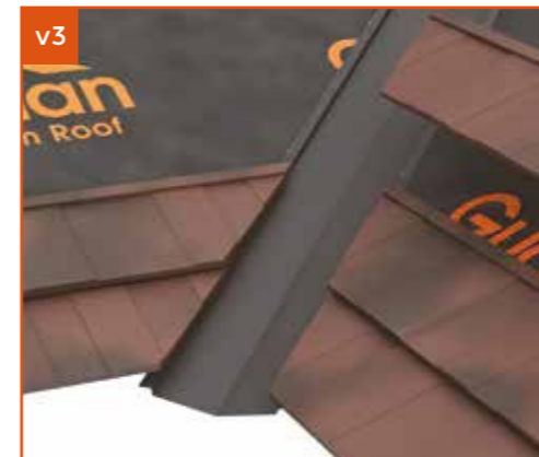
v3 Tile into valley cutting at angle of roof. Seal where necessary.
