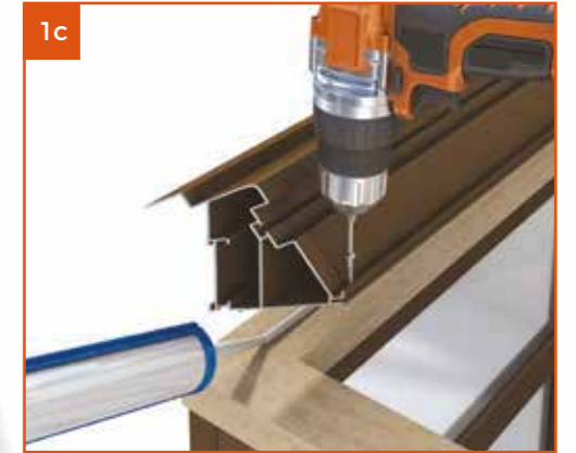
1c Bed ringbeam down on timber packer using low module silicone. Fix ringbeam to timber packer at no more than 100mm from either end then at 500mm centres - using fixings supplied.
