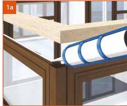
1a Silicone seal 70x60mm timber packer to windows using low module silicone.
