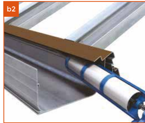
b2 Seal between ringbeam and box gutter with appropriate sealer. Also seal against house wall.
